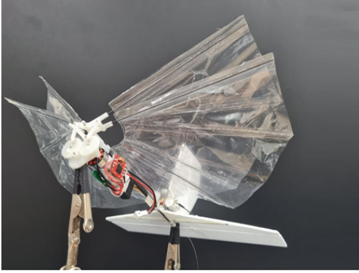
Figure 1: The bio-inspired MAV, CKopter-1.
