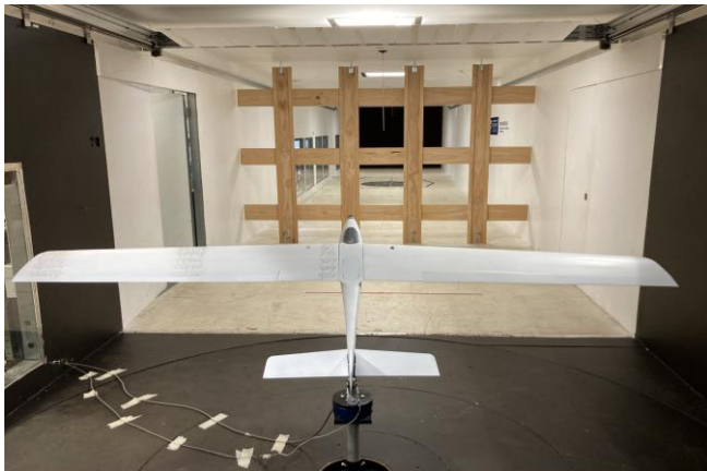
Figure 1: Kahu UAV on load cell, with turbulence grid upstream
