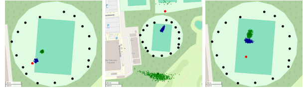
Figure 11: Receiver locations are in black, and the true transmitter location is in red. WCWCL estimates ( g = 1.5 ) are shown in blue, and multilateration estimates ( n = 2 ) in green. The mean estimate location is marked with larger green and blue icons.
