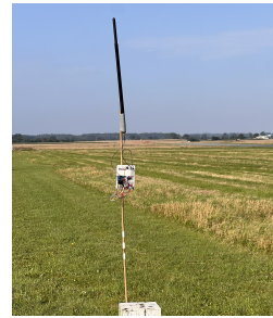
(a) DRID receiver with 9dBi stacked dipole antenna, and SD logging capability.
