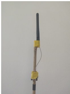
Figure 10: Receiver node with an ESP32-C3 and a 2.15 dBi stacked dipole whip antenna mounted on a bamboo stick, used in the localization experiment.
