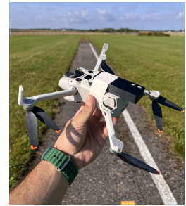
(b) AirPlate DRID emitter mounted underneath the DJI Mini 4 Pro.
