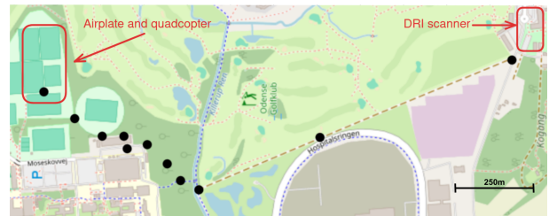
Figure 7: Location of relay nodes used for broadcast mesh network verification. AirPlate[22] and quadcopter are placed on one end of the chain and a DRI scanner on the other end. DRI messages transmitted by the Airplate and quadcopter will be forwarded through the chain of relay nodes using the developed broadcast algorithm.
