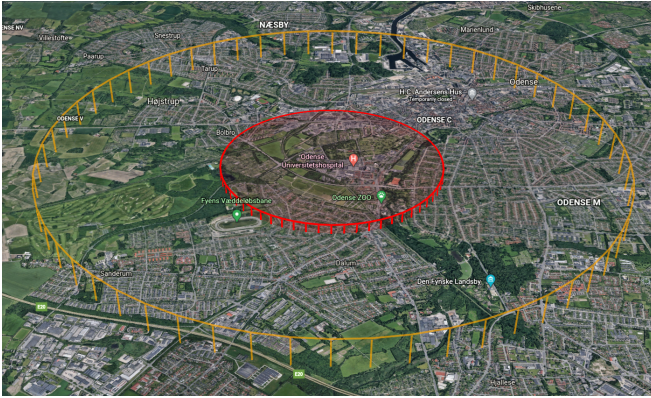
Fig. 4: Illustration of the Detection and Well Clear volumes. The illustration is accurate to scale. The vertical lines are caused by the cylinders being represented by a polygon in this illustration. Map content is Copyright by Google.
