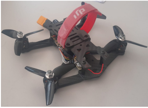
Figure 2: Compact 3-inch quadrotor used for the flight experiments.
