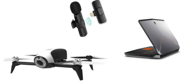
Figure 3: Drone and hardware employed in our experimental framework. We used a wireless microphone transmitting to the GCS, an Alienware 15 R3 laptop.
