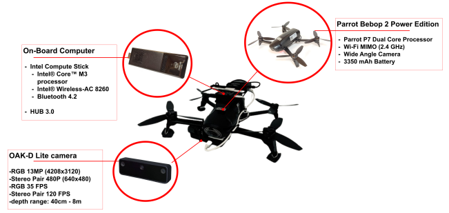
Figure 4: Bebop Parrot 2 with drone equipment specifications.
