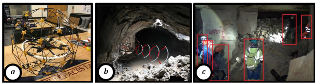
Figure 1: (a) Design for underground applications. (b) Obstacle detection with ultrasound. (c) Detection of workers in mines using the camera [11].
