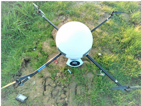
Fig. 3: Multicopter fitted with a 40cm spherical Styrofoam body during mass check right before takeoff.
