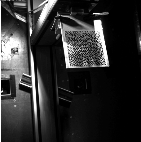
Figure 12: Well-defined aluminum plate with random dot pattern, thickness 8 mm – moved by traversing unit along Z-axis in 25 mm steps
