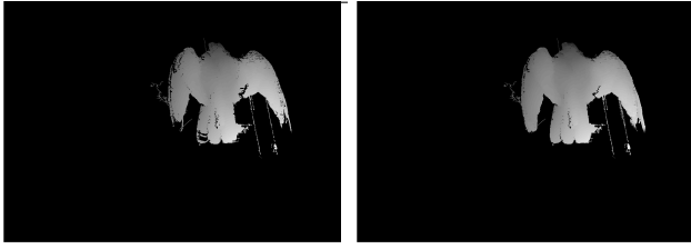
Figure 10: Left image: spatial smoothed disparity map, right image: spatial and temporally smoothed disparity map – gray values from dark gray to white indicate higher disparity and lower depth value – mask is applied to the picture (black background)
